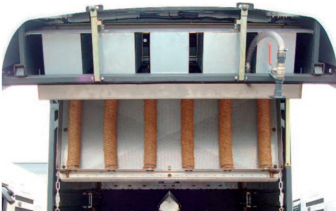
Picture: Water recycling mounted in rear door. Also visible is option 8.5 Sound absorbing damper in rear door
