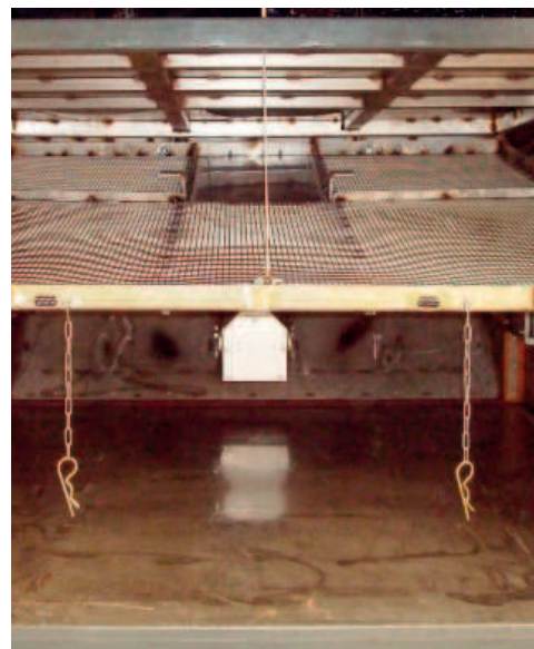
Picture: Mounting rack on the rear of the container and opened Easylift grid
