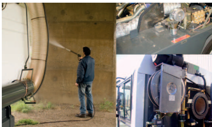
Picture: The high pressure water pump including spray gun and reel
