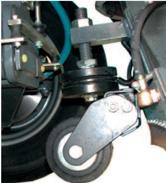
Picture: Suspended swivel wheel and the Hydraulic suction tube shutter
