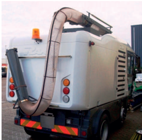
Picture: Wanderhose mounted on rear door and Wanderhose through and mounted on rear door incl. Swasher arm mounted on the Left Hand Side.
