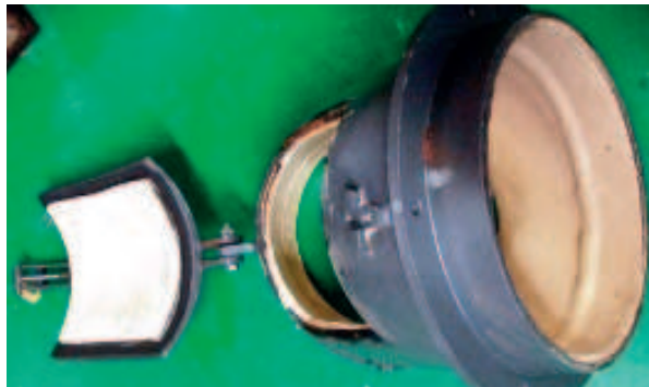
Picture: Coated suction pipe bend in opened and closed position.
