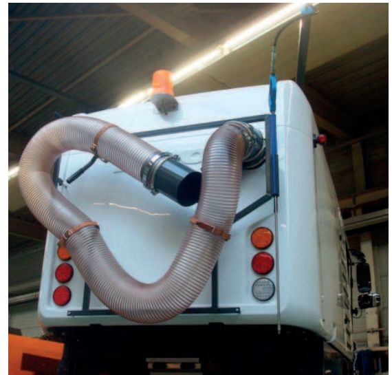
Picture: Wanderhose mounted on rear door and Wanderhose through and mounted on rear door incl. Swasher arm mounted on the Left Hand Side.
