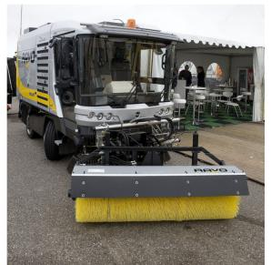
The new RAVO roller brush has been developed by the Dutch RAVO dealer and is available for all RAVO 5-Series units with third brush preparation and quick coupling system.
